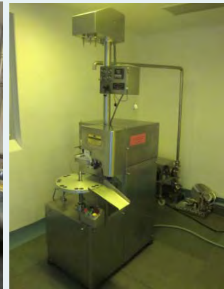
Tube filling equipment used to produce CHX product at Lomus
