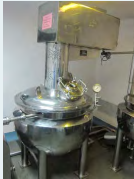
Mixing equipment used to produce CHX gel at Lomus
